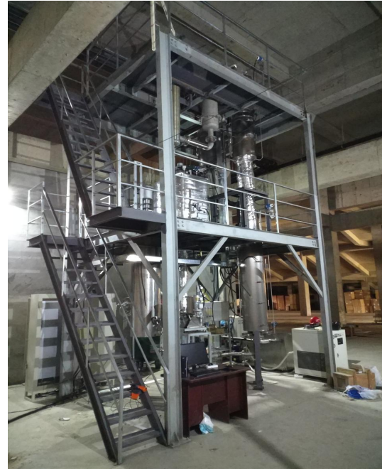
百吨级流化床半干法矿化脱碳中试平台 Hundred tons fluidized bed semi - dry mineralization decarbonization pilot platform
