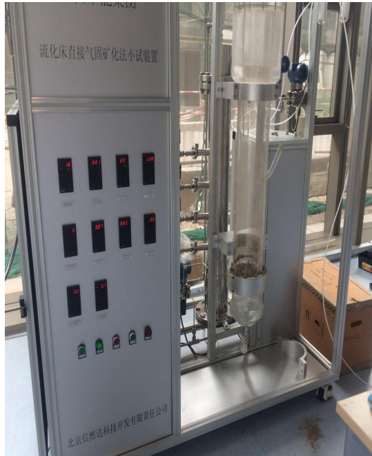
粉煤灰气相矿化法冷态试验研究 Study on cold state test of gas phase mineralization of fly ash
